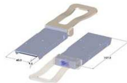
CFP8 transceiver with MPO connector interface
